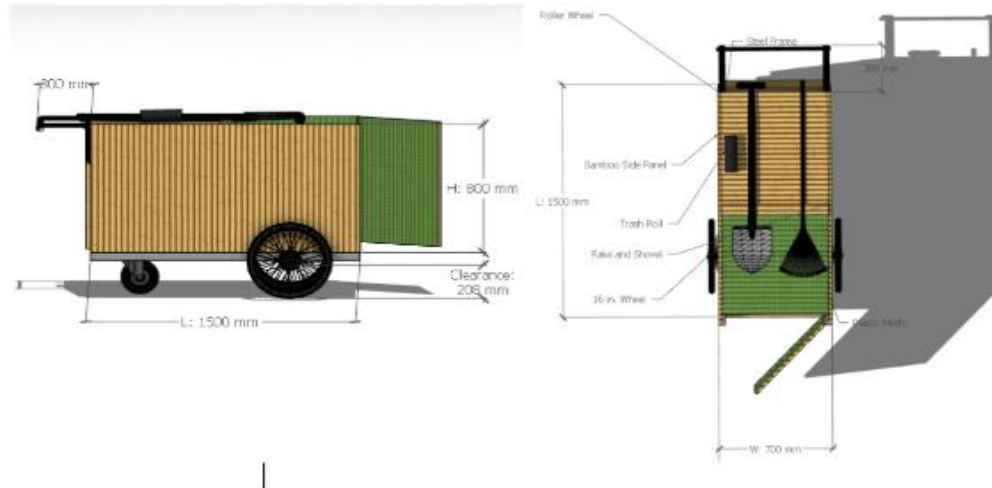
Fig 19. Dimensions of Kariton de Kawayan
